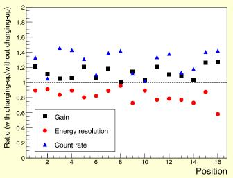
Ratio of gain, energy resolution and count rate after and before the charging-up effect of the Single Mask triple GEM chamber at the sixteen different positions of the chamber. The error bars are smaller than the marker size.
