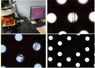
Microscope setup for scanning the GEM foil (top left). Imperfections in the GEM foil at different magnifications (40X: top right, bottom left; 20X: bottom right).
