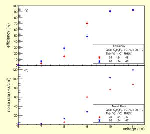
(a) Efficiency as a function of the applied voltage, (b) Noise rate as a function of the applied voltage for  $C_2$   $H_2$   $F_4$  and i- $C_4$   $H_{10}$  gas mixture in 90/10 volume ratio.
