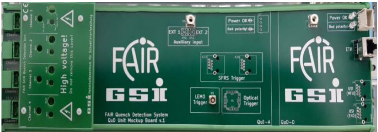
Figure 6: Dummy Quench detection unit
